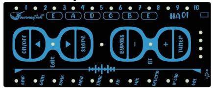
Firstly, press and hold the (on/off ◀ ) button to turn off/on the device.
