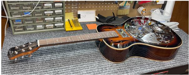
5. After the neck clicks into place in the neck slot, you can pick up the guitar and twist the knob to fully tighten and secure the neck.
